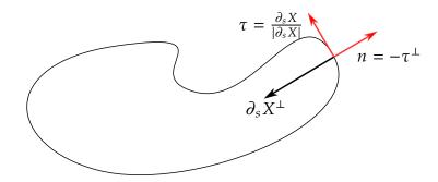
Figure 3: The parameterization and associated vector quantities
