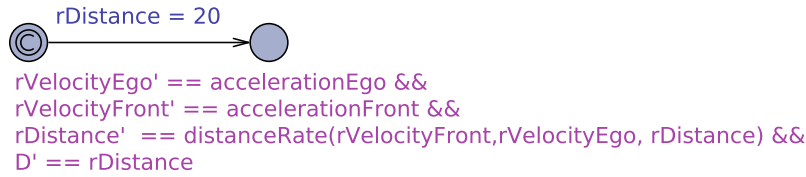
Fig. 8: The monitor component defines a set of differential equation over real variables, these variables can then be used by the learning algorithm.
