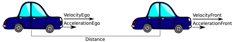
Fig. 2: Distance, velocity and acceleration between two cars [18].
