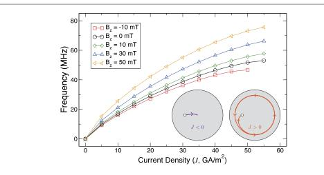
Figure 2. Current dependence of the skyrmion gyration frequency for different perpendicular applied fields,  $B_z$ . An upper critical current density exists at which the skyrmion is expelled from the dot. The inset shows the transient trajectories of the skyrmion core for opposite current polarities.
