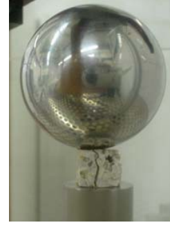
FIGURE 2. Visualization of the experimental set-up based on a Hopkinson bar
