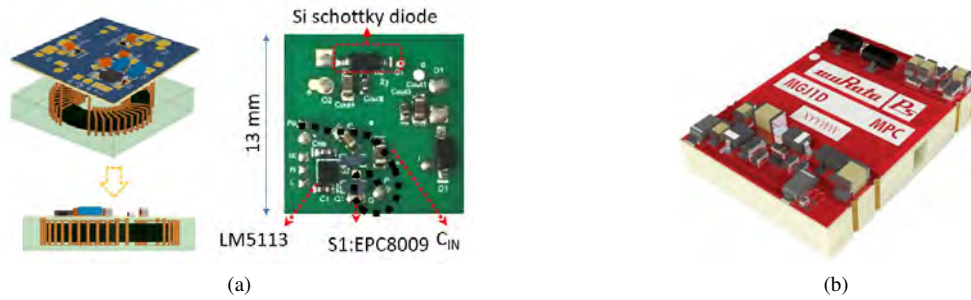
Figure 3: Isolated power supply for gate-drivers. a) Dual output power supply [7]. b) Isolated power supply from Murata [8]
