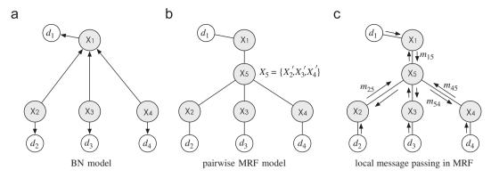
**Fig. 4.** An example of the conversion from (a) a BN to (b) the corresponding pairwise MRF and (c) the local message passing in the MRF. The shaded circles represent the hidden nodes and the white circles denote the observed ones. (a) BN model, (b) pairwise MRF model, and (c) local message passing in MRF.
