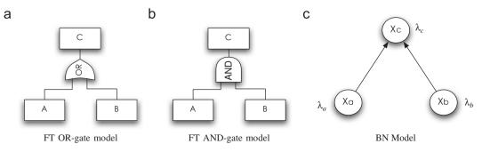
Fig. 1. The simplest OR-gate and AND-gate models described by Fault tree (FT) and Bayesian network (BN). The BN model is converted from the FTs by the method in [15]. (a) FT OR-gate model, (b) FT AND-gate model and (c) BN model.
