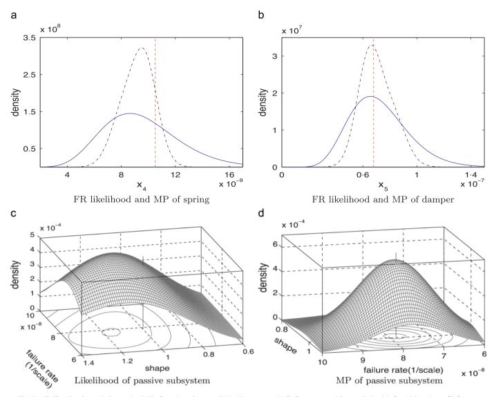
Fig. 10. Likelihood and marginal posterior (MP) of passive subsystem (X<sub>2</sub>) with respect to Weibull parameters (shape and 1/scale) after 10 iterations of inference.
