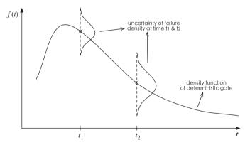
Fig. 2. The stochastic nature of failure density in reliability analysis.
