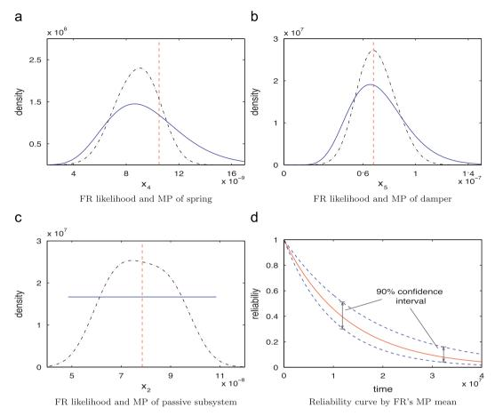
**Fig. 9.** Normalized likelihood and marginal posterior (MP) of FR in the passive subsystem. In (a), (b) and (c) solid lines stand for the likelihoods, dash-dot lines for the posteriors and dashed lines for the actual values. In (d) the solid line represents the reliability of the subsystem by FR's posterior mean and the dashed lines for those of 5% and 95% quantiles of the posterior, indicating the 90% confidence intervals.
