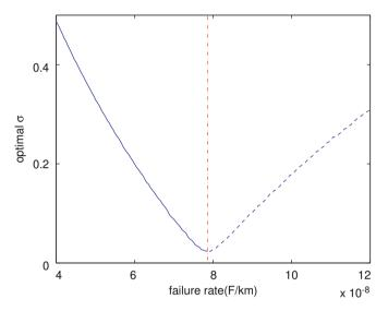
**Fig. 8.** Monte Carlo simulation of learning  $\sigma$  in Eq. (6), where  $X_4 = 0.105 \times 10^{-7}$  F/km,  $X_5 = 0.68 \times 10^{-7}$  F/km.
