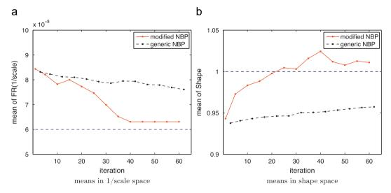
Fig. 11. Scale and shape means of system Weibull model in 60 iterations by the NBP and the modified NBP algorithm. The dashed lines denote the actual values.
