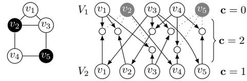
■ **Figure 2** **Left:** A graph with its dominating set in black. **Right:** The corresponding instance and 2-orientation, where deleted vertices are in gray. Original edges with a deleted vertex as an endpoint are dotted.
