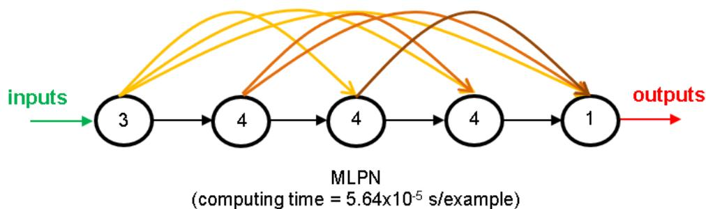
**Fig. 4** Proposed 3-4-4-4-1 fully-connected MLPN – simplified scheme.
