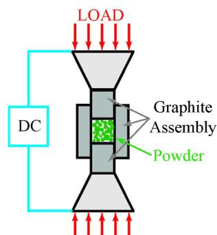
Figure 3.3 - Schematic set-up of the SPS technology.
