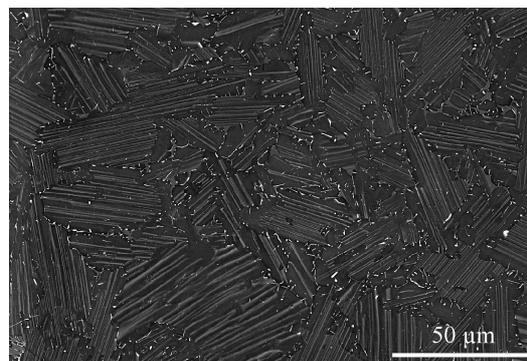
Figure 3.5 - Typical microstructure of the IRIS alloy ; the borders of the lamellar colonies are composed of black  $\gamma$  phase and white B2 phase.
