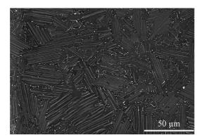
Figure 3.5 - Typical microstructure of the IRIS alloy; the borders of the lamellar colonies are composed of black γ phase and white B2 phase.
