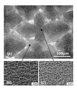
Figure 2.2 - Dendritic microstructure of the as-cast MC-NG SC superalloy normal to the <001> growth direction: (a) at the dendrite scale, imaged by light microscopy (LM); (b) and (c)  $\gamma'$  precipitates, imaged by scanning electron microscopy (SEM).
