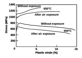
Figure 2.7 - Effect of an air exposure for 200 hours at 1050°C and 80 MPa on the engineering stress-strain tensile curves at 650°C and 950°C of <001> MC2 single crystals.
