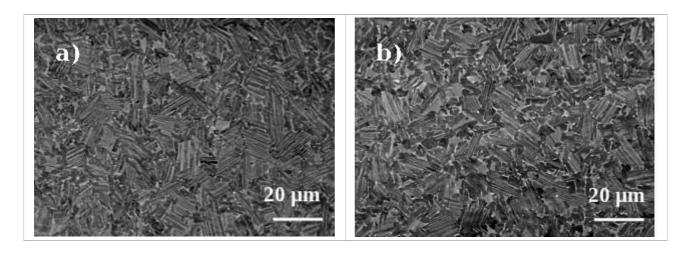
Figure 3.4 - Fine-grained fully lamellar microstructures obtained for a) SPS at 1190°C, b) SPS at 1250°C.
