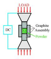
*Figure 3.3 - Schematic set-up of the SPS technology.*
