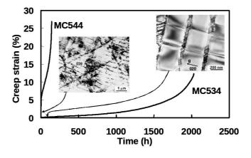
Figure 2.5 - Creep behaviour and deformation mechanisms at 760°C and 840 MPa of MC544 and MC534 <001> single crystal specimens.
