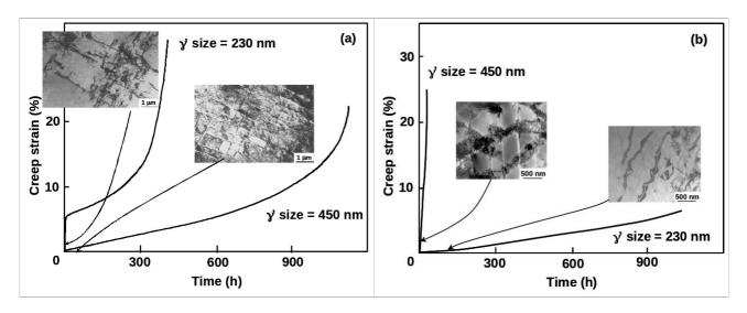
Figure 2.4 - Effect of the  $\gamma'$  precipitate size on the deformation mechanisms and creep behaviour at 760°C and 750 MPa of CMSX-2 SC superalloy along: a) <001>; b) <111>.
