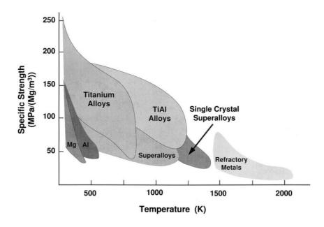
*Figure 3.1 - Temperature capabilities of different classes of materials.*
