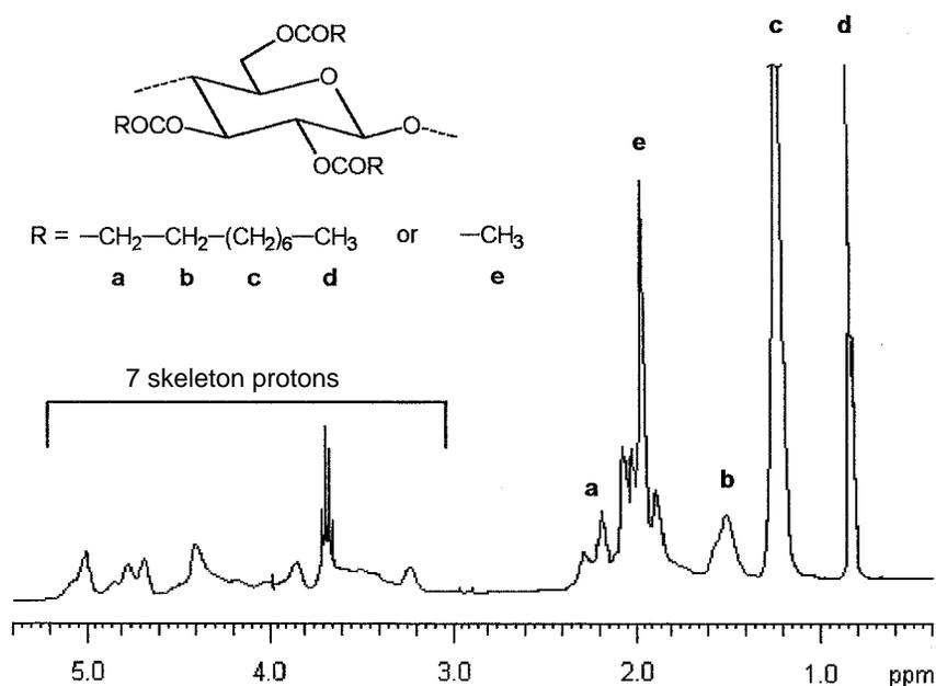
**FIG. 1.** Proton nuclear magnetic resonance spectrum of cellulose mixed acetic-decanoic triester in CDCl<sub>3</sub> (DS<sub>acetyl</sub> = 2.18; DS<sub>decanoyl</sub> = 0.82). DS, degree of substitution.
