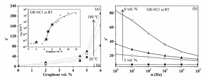
Fig. 6. (a) Real part of the dielectric permittivity versus graphene vol% for PEKK and PEKK/"as received" graphene (GR-NC1) at (■) 20 °C, (○) 160 °C and (▲) 180 °C. Inset: DC conductivity versus GR content at room temperature. (b) Real part of the dielectric permittivity versus frequency for PEKK and PEKK/"as received" graphene (GR-NC1) at room temperature: (■) 2 vol% graphene, (○) 4.5 vol% graphene, (▲) 5 vol% graphene and (▽) 6 vol% graphene. Solid lines are guide for the eve.
