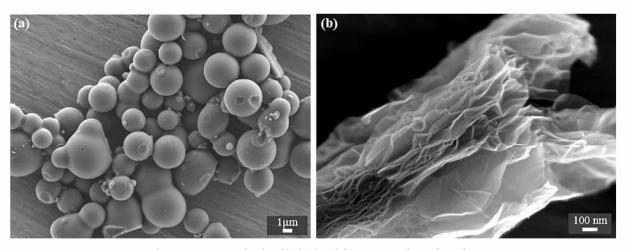
Fig. 1. SEM images of carbon black (a) and the "as received" graphene (b).
