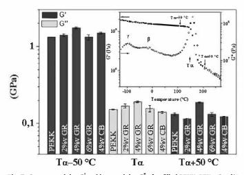
Fig. 7. Storage modulus G and loss modulus G of unfilled PEKK, PEKK/2 vol% GR, PEKK/4 vol% GR, PEKK/6 vol% GR and PEKK/4 vol% CB, measured at  $T\alpha - 50$  C,  $T\alpha$  and  $T\alpha + 50$  C. Inset: PEKK matrix thermogram between -130 °C and 270 °C.
