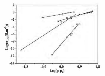
Fig. 4. Power law fit for GR-NC1 ( $\square$ ), GR-NC2( $\bigcirc$ ), GR-NC3 ( $\triangle$ ) and CB-NC ( $\bigcirc$ ). Solid line is the linear fit.
