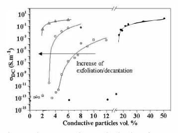
**Fig. 3.** DC conductivity versus conductive particles volume fraction for GR-NC1 ( $\Box$ ), GR-NC2 ( $\bigcirc$ ), GR-NC3 ( $\triangle$ ) and CB-NC ( $\bigcirc$ ). Solid line is the percolation threshold fit.
