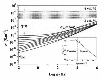
Fig. 5. Real part of the conductivity versus frequency for PEKK/home-exfoliated graphene (GR-NC2) 3 vol% (solid line) and 4 vol% (dashed line) for isotherms from -150°C to 200 °C.
