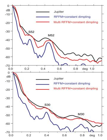
**Fig. 7.** Effect of multi-moding, which increases the level of grating lobes at 857 GHz, making it close to the measured ones. Two stacked cuts are shown to enhance the visibility of the main grating lobes (*top panel*: cuts at  $\pm 26^{\circ}$ , *bottom panel*: cuts at multiples of  $60^{\circ}$ ). In blue is shown the single-moded RFFM plus constant dimpling fit at 353 GHz, and in red the equivalent multi-moded model, while the measurements on Jupiter are in black.
