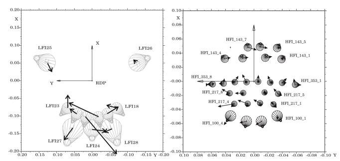
Fig. 18. Left panel: displacement residuals remaining on LFI detectors after removing the joint fit. Right panel: residuals remaining on HFI detectors after removing the joint fit. The axis units are mm.
