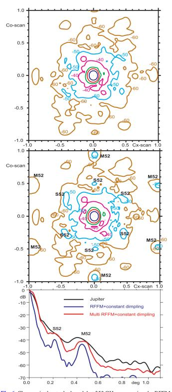
**Fig. 6.** Changes in the stacked model at 353 GHz, comparing the RFFM (*top panel*) to the RFFM, with the addition of a best-fit constantdimpling model (*centre panel*). The cut (*bottom panel*) is a stack of cuts at  $\pm 16^{\circ}$  to enhance the M52 and S52 lobes. The amplitude of the S30 lobes (not shown) is hardly enhanced by the additional dimpling.
