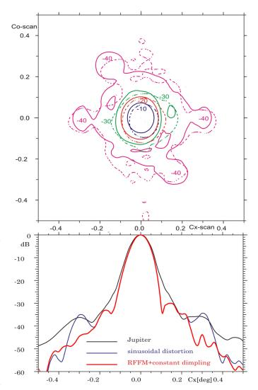
**Fig. 9.** Model with three sinusoidal deformations of the subreflector at 353 GHz. This yields a good fit to the lobes located  $0.3^{\circ}$  from beam centre. We compare here the RFFM + constant dimpling model with and without the addition of these deformations. The *top panel* shows the measured Jupiter map in dashed contours.
