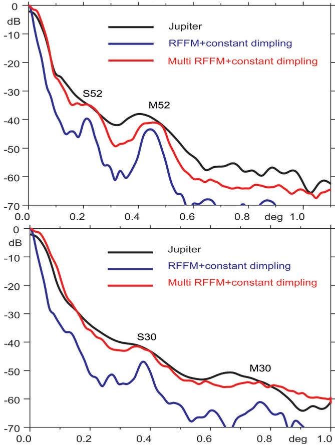
**Fig. 7.** Effect of multi-moding, which increases the level of grating lobes at 857 GHz, making it close to the measured ones. Two stacked cuts are shown to enhance the visibility of the main grating lobes (*top panel*: cuts at  $\pm 26^\circ$ , *bottom panel*: cuts at multiples of  $60^\circ$ ). In blue is shown the single-moded RFFM plus constant dimpling fit at 353 GHz, and in red the equivalent multi-moded model, while the measurements on Jupiter are in black.
