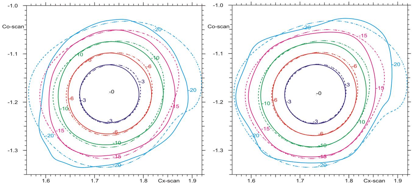
**Fig. 17.** *Left panel:* comparison of fsbeam of detector 143-5 (full line) to the retrieved model (dashed line). *Right panel:* comparison of Mars-based beam of detector 143-5 (full line) to the retrieved model (dashed line). The Mars-based beam shows extended modelled shoulders that are not present in fsbeam, but are present in the model beam. The inference is that the use of fsbeam introduces non-optical features in the beam.
