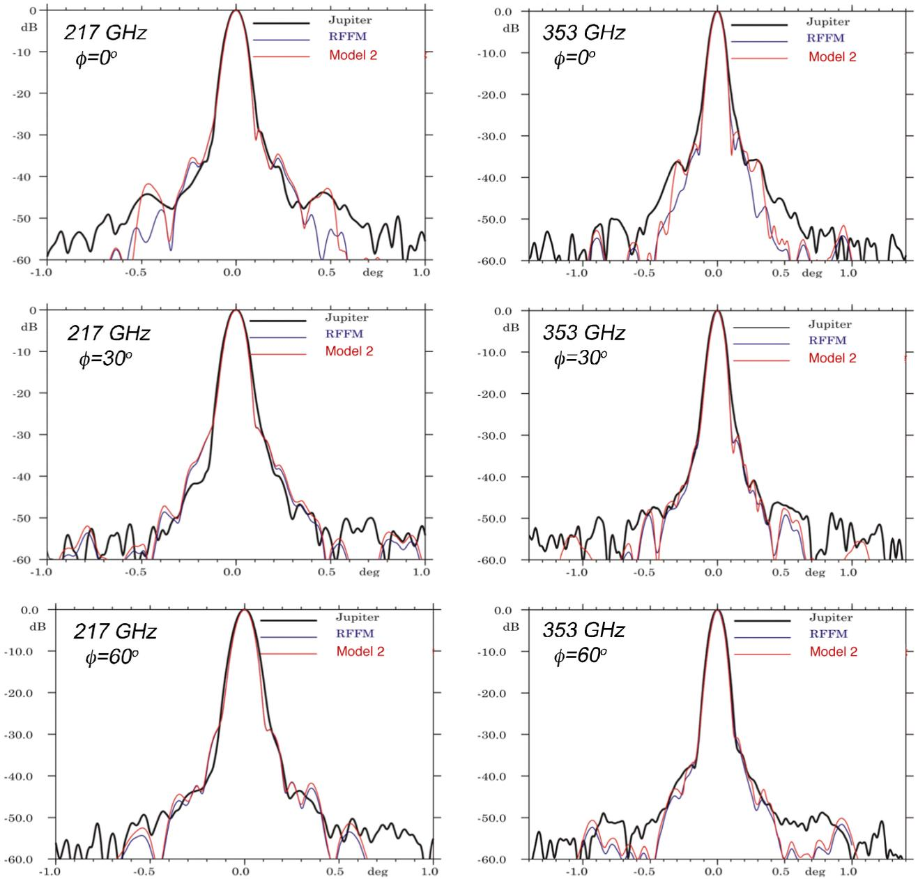
**Fig. 12.** Three radial cuts, at  $\phi = 0^\circ$ ,  $30^\circ$ , and  $60^\circ$ , from the cross-scan directions. The curves show the measured pattern (black), the RFFM (blue), and Model 2 (red). 217 GHz is shown on the *left* and 353 GHz on the *right*.
