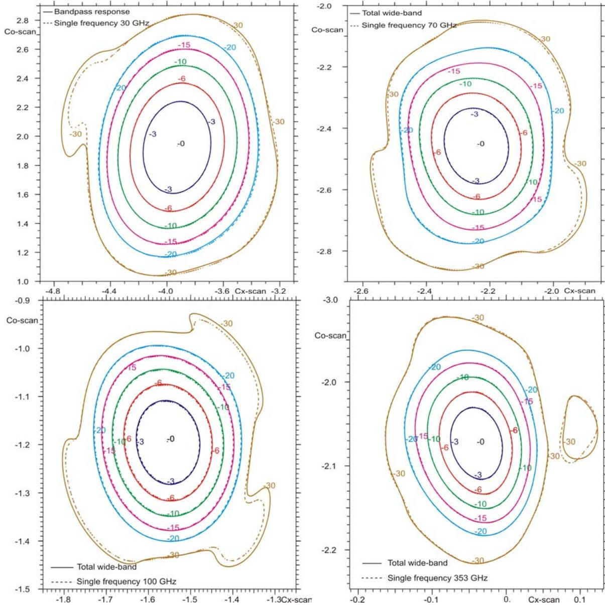
**Fig. 15.** Difference in predicted patterns between monochromatic and wideband models. The four detectors shown are 27S (30 GHz), 18S (70 GHz), 1a (100 GHz), and 1 (353 GHz). The bandpass shape is realistic and the source spectrum assumed here is CMB (but a similar result is obtained when the source spectrum assumed is that of Mars). In this and all subsequent beam contour plots, the axis units are in degrees.
