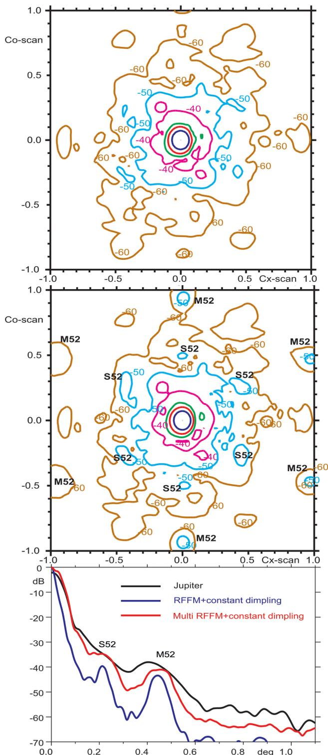
**Fig. 6.** Changes in the stacked model at 353 GHz, comparing the RFFM (top panel) to the RFFM, with the addition of a best-fit constant-dimpling model (centre panel). The cut (bottom panel) is a stack of cuts at  $\pm 16^\circ$  to enhance the M52 and S52 lobes. The amplitude of the S30 lobes (not shown) is hardly enhanced by the additional dimpling.
