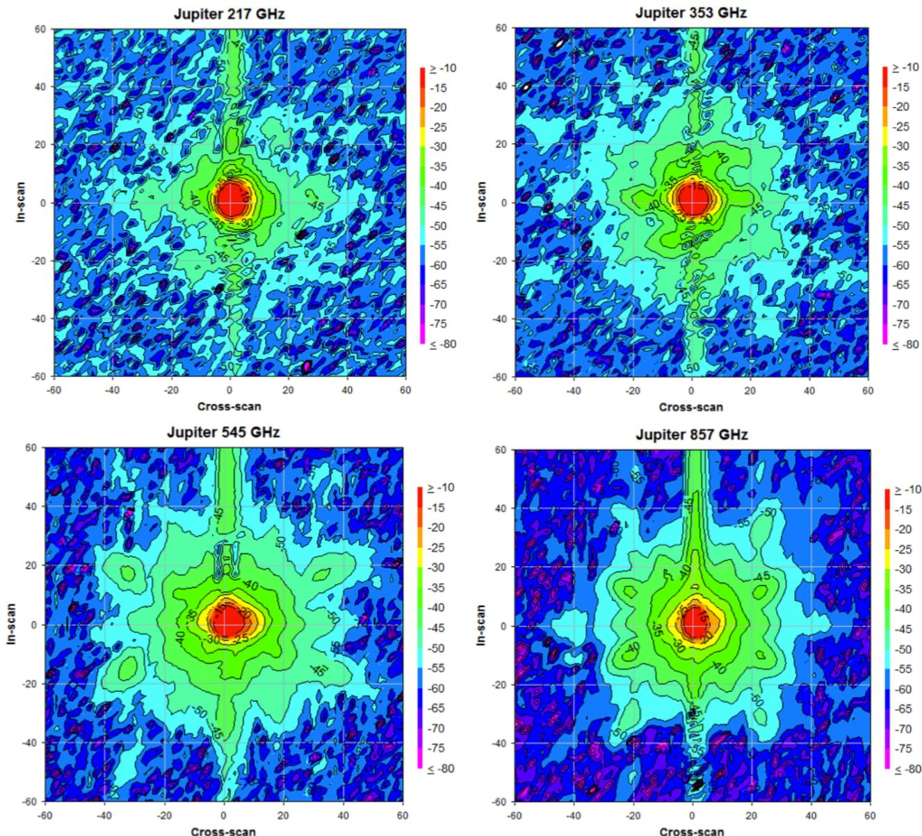
**Fig. 4.** Stacked observations of Jupiter for the frequencies 217–857 GHz. Here “stacked” means that all available Jupiter maps at a given frequency (from individual detectors and individual planet passes) are averaged together. The coordinate axes are in arcminutes.
