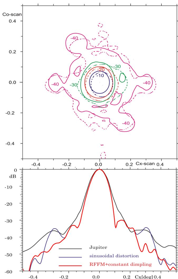
**Fig. 9.** Model with three sinusoidal deformations of the subreflector at 353 GHz. This yields a good fit to the lobes located  $0.3^\circ$  from beam centre. We compare here the RFFM + constant dimpling model with and without the addition of these deformations. The *top panel* shows the measured Jupiter map in dashed contours.
