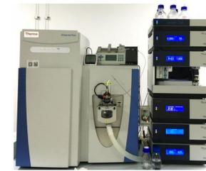
Acquisition of mass spectra using a LC/MS/MS (capLC-QexactivePlus(thermofisher scientific)).
