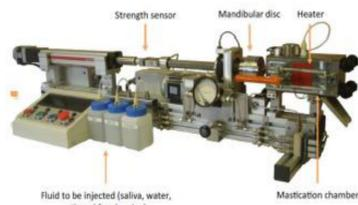
**In vitro gastric digestion using a dynamic artificial digestive system: DIDGI® (INRA, GPMA, France)**
