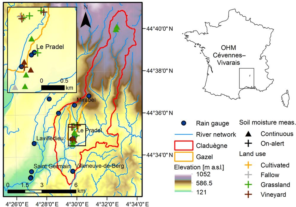
**Figure 1.** Location of the study site and measurement network. At every on-alert site measurements were taken at about 10 randomly chosen locations. At every continuous measurement sites two sensors were installed at 10 cm depth, two sensors at 20–25 cm depth and one sensor at a depth of 33–50 cm.
