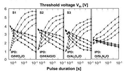
Fig.4 Program erase characteristics of Si-nc memories with various O/high-k/O IPD stacks (WxL=0.5 \mu mx0.25 \mu m). V<sub>P</sub>: 14V to 17V. V<sub>E</sub>: -12V to -15V.
