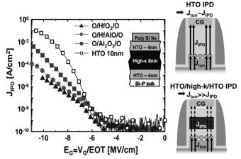
Fig.3 Leakage currents of 3-layer interpoly capacitors. Different O/highk/O stacks are measured, HTO reference is also represented. On the right: schematics of the filling and emptying currents during writing.
