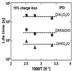
Fig.11 Life time vs measurement temperature for samples S1 to S3
