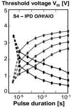
Fig.5 Program erase characteristics of sample S4. V<sub>P</sub>: 10V to 13V. V<sub>E</sub>: -11V to -13V.
