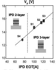
Fig.7 Program voltage required for a  $\Delta V_{th}$  of 2.5V with 1ms pulses, vs IPDs EOT. Different 3-layer and 2layer IPD are shown.
