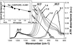
Fig.2 Infrared spectra of 6nm ALD deposited HfAlO films of various Hf:Al compositions. Inset: measured optical bandgap (ellispometry) vs the Hf fraction of HfAlO alloys.
