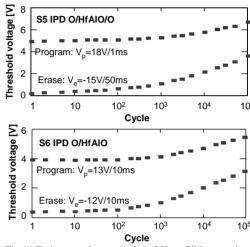
Fig.14 Endurance characteristics of Si-nc/SiN memories with 3-layer (S5) and 2-layer (S6) IPDs.
