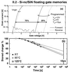
Fig.13 (a) Id(Vg) in forward (Vd=1.5V) and reverse (Vd=-1.5V) modes for S5. (b) Normalized retention curves of the programmed states of S5 ( $\Delta V_{th}$ =3.5V).
