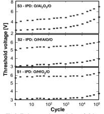
Fig.8 Endurance characteristics of 3-layer IPD memories (S1 to S3), with various O/high-k/O IPDs. Program: V<sub>P</sub>=18V/1ms, erase: V<sub>E</sub>=-15V/1ms.
