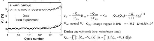
Fig.16 Simulated endurance characteristics for S1, assuming a progressive trapping in the middle of the IPD stack during cycling, modelled by an empirical law [9]. v=-0.2, K=6.35.10<sup>-7</sup>.
