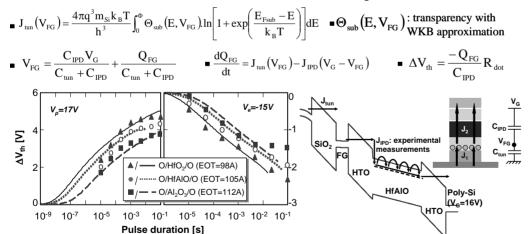
Fig.15 Simulated program/erase characteristics. Lines: simulations (Si-ncs area coverage [8]:  $R_{dot}$ =50%), symbols: data. In high-k IPD memories, as  $J_{IPD}$ << $J_{tun}$ , the memory window is essentially controlled by the IPD EOT.
