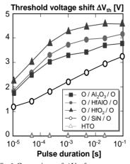
Fig.6 Comparison of  $\Delta V_{th}$  for a program voltage of 18V for memory devices with various 3-layer IPDs. Control devices with ONO and HTO IPD are also shown
