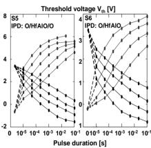
Fig.12 Program erase characteristics of Sinc/SiN memories (S5 and S6). S5:  $V_p$ : 14V to 18V.  $V_e$ =-12V to -15V. S6:  $V_p$ : 10V to 13V.  $V_e$ =-10V to -13V.  $W_x$ L=0.5 $\mu$ mx0.25 $\mu$ m.
