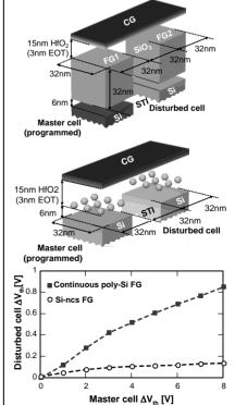
Fig.17 TCAD 3D simulation of the FG/FG cross coupling in a poly-Si FG memory and in a Si-nc memory.  $\Delta V_{th}$  is analytically calculated from the simulated FG potentials.
