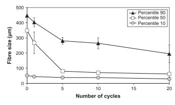
Fig. 5. Evolution of the wood fibres size distribution versus the number of cycles after dissolution of the composite matrix in THF, filtration of the fibres and drying.
