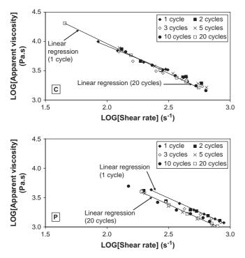
Fig. 1. Evolution of the apparent viscosity versus the shear rate for the composite  $(\mathbf{C})$  and the polymer  $(\mathbf{P})$ .
