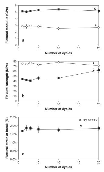
Fig. 2. Evolution of the flexural properties versus the number of cycles for the polymer  $(\mathbf{P})$  and the composite  $(\mathbf{C})$ . (a) Flexural modulus; (b) flexural strength; (c) flexural strain at break.
