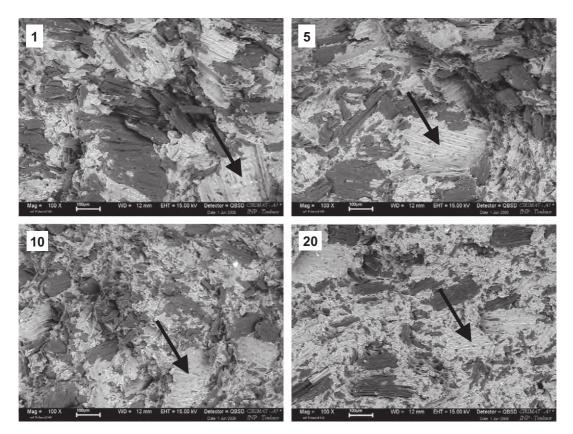
Fig. 4. Micrographs (100×) of the impact test fracture surface of the composite samples (C) after 1, 5, 10 and 20 cycles. Black arrows highlight the debonding zones.
