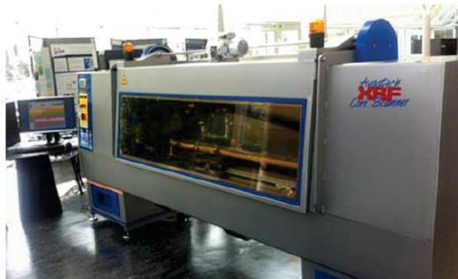
Figure 9. Core-scanner Optical XRF Avaatech (Source : Avaatech)
