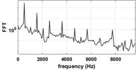
Figure 17 - FFT of lift from the URANS simulation
