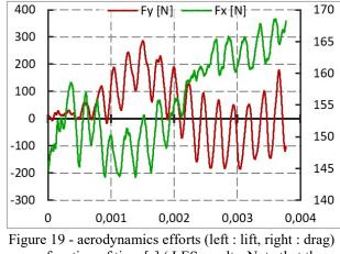
as a function of time [s] ( LES results. Note that the transient phase of the computation is still not fully completed, as only the first buffeting period has been computed yet)
