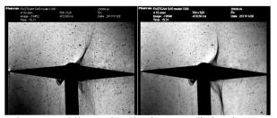
Figure 6: Schlieren visualizations at 2 distinct instants, revealing the oscillations of the shock waves associated with the buffeting phenomenon
