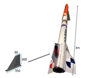
Figure 1 - Global view of the SERA launcher and details of the aileron shape and dimensions [mm]
