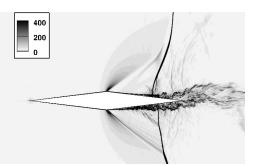
Figure 10 - Instantaneous flow fields coloured with the density gradient, showing dissymmetric shock waves (wall-model LES)
