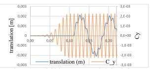
Figure 25 – Fluid / structure coupled simulation, showing the displacement of the airfoil (red) due to aerodynamic forces (blue)
