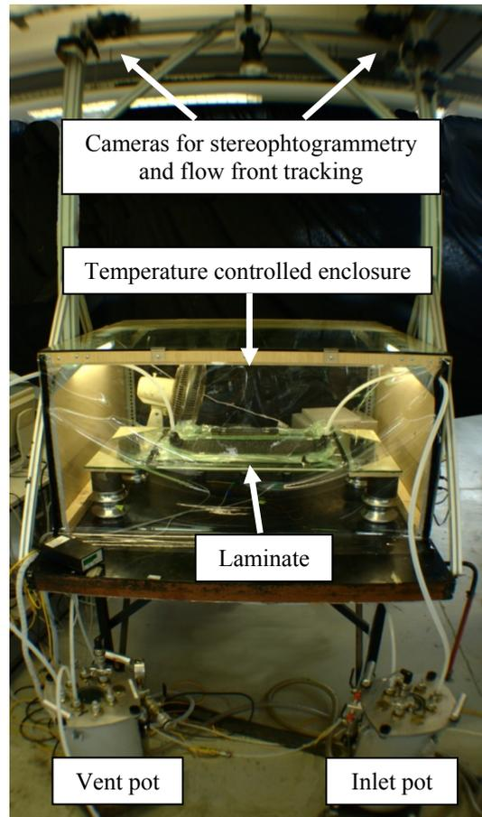
Fig. 3: Experimental setup for monitoring resin infusion.
