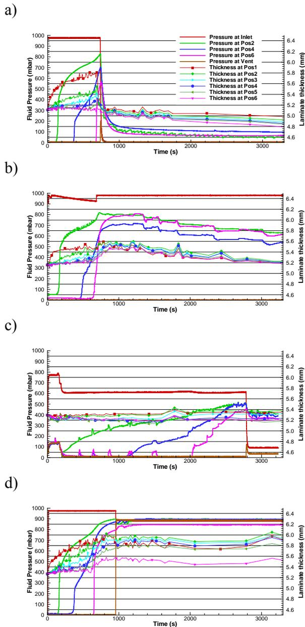
Fig. 5: Traces of the fluid pressure and laminate thickness for four experiments; a) EQ A/0(r3), b) EQ A/C(r2), c) EQ 650/0, and d) EQ A/900(r3).
