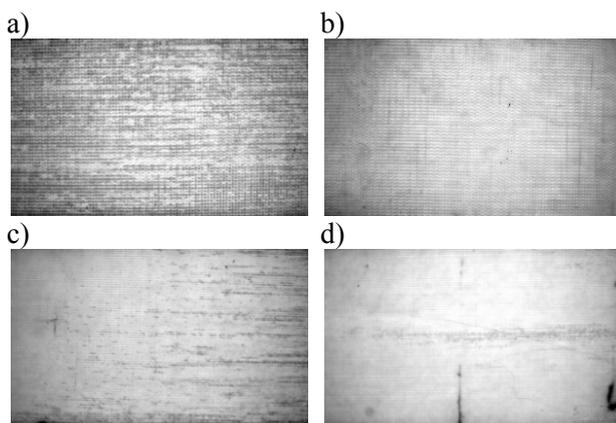
Fig. 6 Pictures of light transmitted through manufactured panels; a) EB-A/0 (r2), b) EB-A/C, c) EQ-A/900 (r1), and d) EQ-A/900 (r2).
