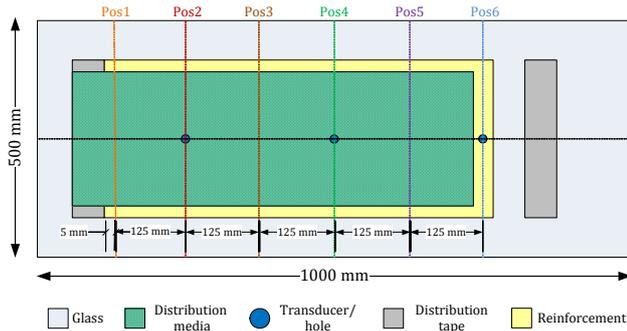
Fig. 4: Schematic of the laminate and consumables layout.
