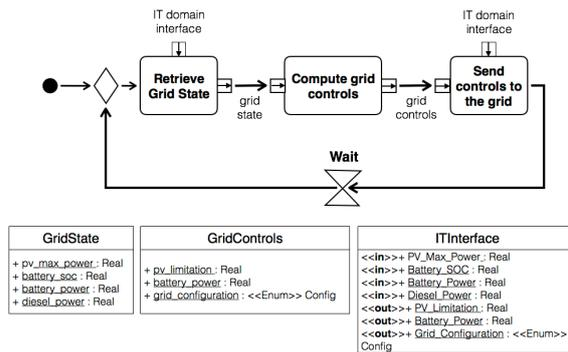
Figure 3: Use case: *IT process model* in fUML
