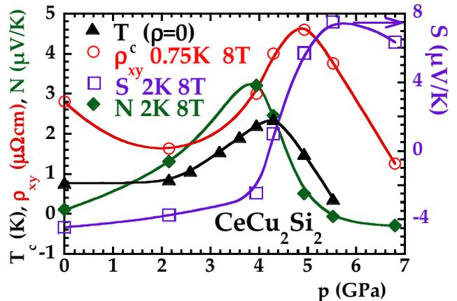
FIG. 3.  $p$ -dependence of  $T_c^{\rho=0}$ ,  $\rho_{xy}(0.75 \text{ K}, 8 \text{ T})$ ,  $S(2 \text{ K}, 8 \text{ T})$  and  $N(2 \text{ K}, 8 \text{ T})$  (lines are guides to the eye). The maximum  $T_c$  is accompanied by a pronounced peak in  $N(p)$  and a signchange in  $S(p)$ , whereas the maximum in  $\rho_{xy}(p)$  occurs at slightly higher  $p$ , more following  $\rho_0(p)$  (see fig. 5b).
