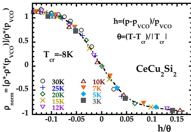
FIG. 7. Best collapse of all normalized  $\rho_{\text{norm}}(p)$  data (from fig. 6a) as a function of the generalized “distance”  $h/\theta$  from the CEP ( $T_{cr} \sim -8$  K,  $p \geq 3.6$  GPa, dashed line: guide to the eye). Within the universal framework of critical phenomena (see text), such a representation corresponds to  $\gamma = 1$  and  $\delta \rightarrow \infty$ .
