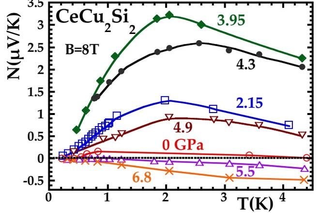
FIG. 12.  $T$ -dependence of the NERNST signal  $N(8\text{ T})$  at several  $p$  up to 6.8 GPa. As a function of  $p$ , the NERNST signal first increases, with a maximum at 4 GPa (see fig. 3), before decreasing again and even switching to negative values at high  $p$ . Below 5 GPa, a characteristic energy scale may be revealed through the maximum in  $N(T)$  around 2 K. (lines are guides to the eye only)
