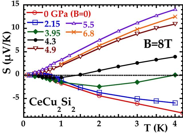
FIG. 11.  $T$ -dependence of the thermoelectric power  $S(8\text{ T})$  at several  $p$  up to 6.8 GPa. Remarkably, a sign change from negative to positive takes place around 4 GPa within the entire investigated  $T$  range. For  $0 < p < 5$  GPa,  $S(8\text{ T})$  remains negative down to the lowest available  $T$ . The  $p$ -dependent sensitivity on magnetic field is displayed in figs. 14a-c. (lines are guides to the eye only)
