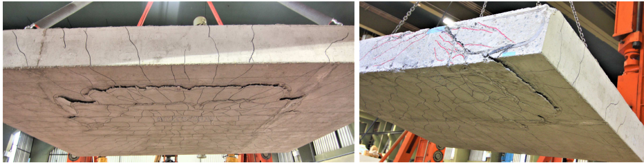
Figure 3 : Thick slab failure mode: a) bottom face; b) saw-cut
