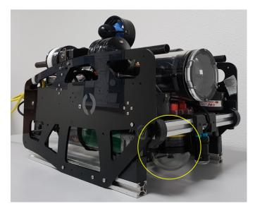
Fig. 7: AUV with downward-looking camera (inside yellow circle)
