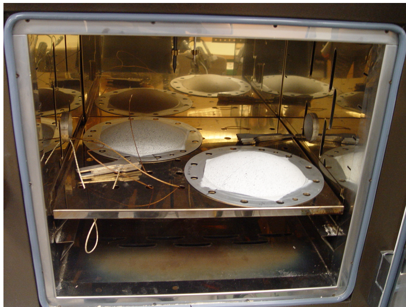
Figure 3. Thermal treatment of bulged specimen.
