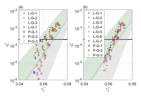
Figure 11: Evolution of the dimensionless bedload rate with dimensionless skin friction: (a) rising and (b) falling limbs data. Gray and green shaded areas are the same as in Figure 6. Black horizontal line corresponds to  $q_{s-\text{ref}}^* = 2.2 \times 10^{-4}$ .
