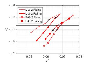
Figure 7: Bedload hysteresis patterns for L-G-2 and P-G-2. Black arrows indicate the hysteresis direction. Black horizontal line corresponds to  $q_{s-\text{ref}}^* = 2.2 \times 10^{-4}$ . The bedload rates presented here correspond to values averaged over each steady plateau.
