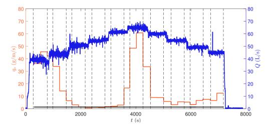
Figure 9: Time variations of bedload rates (in orange) and flow (in blue); results for the H-G/S-7 test. Grid delimits steady states from transition zones. Black horizontal line corresponds to  $q_{s-\text{ref}} = 1.325 \text{ g.m}^{-1} \text{.s}^{-1}$ .
