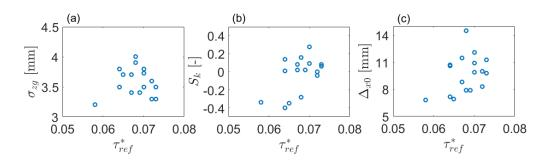
Figure 12: Relation between dimensionless reference bed shear stresses and their associated bed surface indicators. Bed surface parameters are (a) geometrical grain roughness or (b) bed armoring degree or (c) the length of the bed surface structures in the flow direction.
