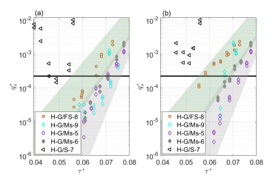
Figure 8: Evolution of the dimensionless bedload rate with dimensionless bed shear stress; results for infiltrated gravel beds: (a) at the rising limb and (b) at the falling limb. Green and grey shaded areas are the same as presented in Figure 6. The open and closed symbols denote data obtained on hybrid beds resulting from initial loose and packed beds, respectively. Black horizontal line corresponds to  $q_{s-\text{ref}}^* = 2.2 \times 10^{-4}$ .
