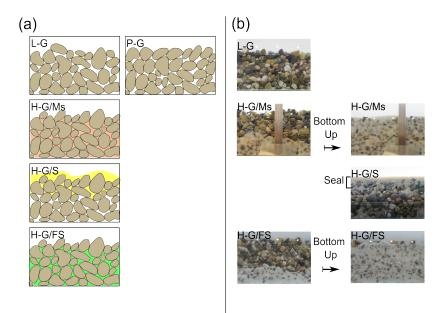
Figure 3: (a) Diagrams illustrating the beds studied and (b) lateral photographs of the beds during (left) and at the end (right) of the infiltration phase.
