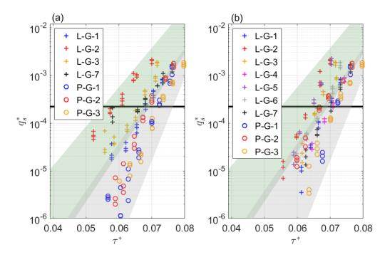
Figure 6: Evolution of the dimensionless bedload rate with dimensionless bed shear stress; results for the clean L-G and P-G beds: (a) at the rising limb and (b) at the falling limb. Green and grey shaded areas delimit loose bed data and packed bed data, respectively, during the rising limb. These areas are reported on Figure 6b. Black horizontal line corresponds to  $q_{s-\text{ref}}^* = 2.2 \times 10^{-4}$ .
