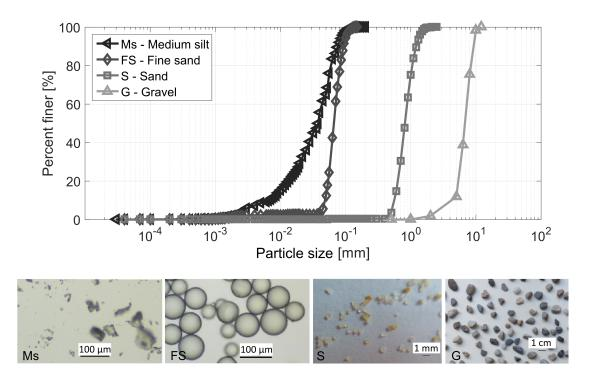
Figure 2: Sediment GSD and shapes. Photographs of Ms and FS were taken with a microscope.
