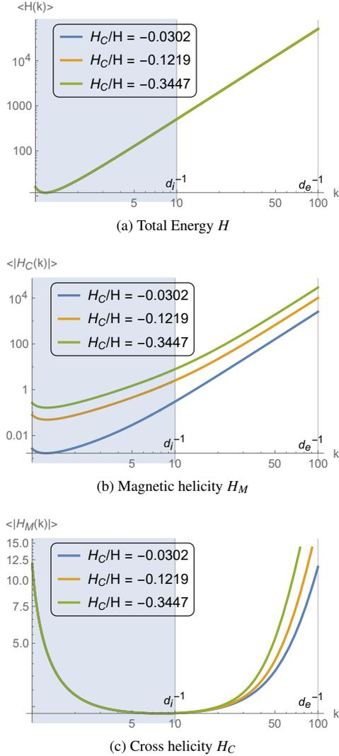
FIG. 5. Log-Log Plots for total energy, magnetic and cross-helicity. The parameters used here are  $\alpha = 10$ ,  $\beta = 9$  and  $\gamma = \{0.001, 0.03, 0.1\}$  is varied so that different values of  $H_C$  are obtained (color-coded, see the legend for the description). The microscales were chosen to be  $d_i = 0.1$  and  $d_e = 0.01$ .
