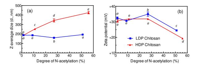
**Figure 2.** Variation of a) Z-average size and b) Zeta potential of chitosan-pentasodium tripolyphosphate (CS-TPP) nanoparticles, isolated and re-suspended, with the degree of acetylation of chitosan of low degree of polymerization (DP~58-82) and of high degree of polymerization (DP ~ 776 - 1442) degree of polymerization (as indicated in legend; CS:TPP mass ratio was fixed to 4:1; water; mean average values  $\pm$  SE; different letters in symbols denote significant differences p≤0.05, *n*=3).
