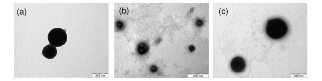
**Figure 3**. TEM micrographs of chitosan–TPP nanoparticles prepared from chitosan of varying  $M_w$  and DA: a) LDP DA 9.2%; b) HDP DA 11% and c) HDP DA 56%. The nanoparticles were stained with phosophotungstic acid 2 % (w/w).
