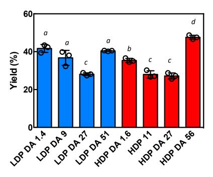
**Figure 1.** Production yield of chitosan–TPP nanoparticles as a function of chitosan's degree of N-acetylation of low ( $M_w \sim 10$  kDa) and high (Mw $\sim 120$  kDa) degree of polymerization (as indicated in legend; CS:TPP mass ratio was fixed to 4:1; water) (mean average values ± SE; different letters in symbols denote significant differences among treatments p $\leq 0.05$ ; n=3).
