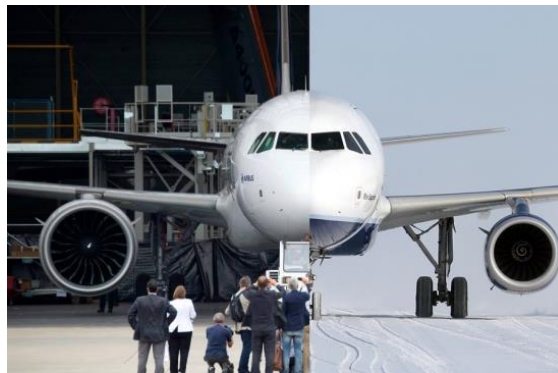
Figure 2: Illustration of the limited margins for further increase of fan diameter on Small-Medium Range airplanes 12
