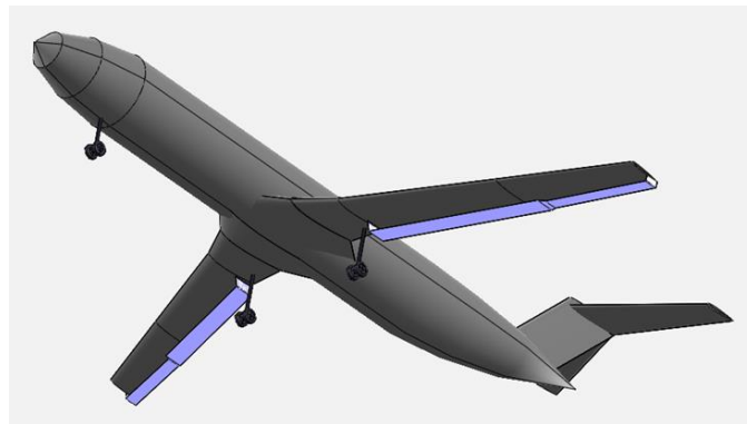
Figure 7: DRAGON landing gear layout and distributed fans location
