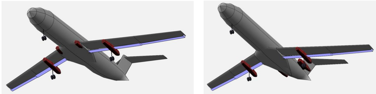
Figure 6: Configuration exploration with podded landing gears at the rear of under the wing turboshafts
