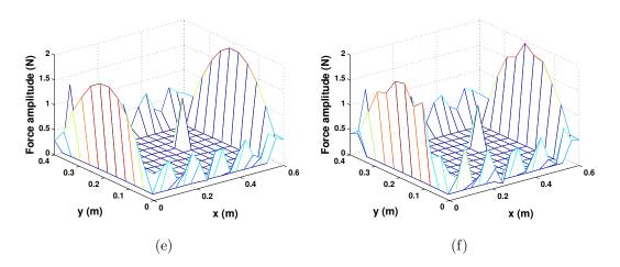
Figure 7: Identification of the force vector  $\mathbf{\mathcal{F}_{m}}$  at resonance frequencies of the structure - (a) Reference at 378 Hz, (b) Identification at 378 Hz, (c) Reference at 720 Hz, (d) Identification at 720 Hz, (e) Reference at 915 Hz and (f) Identification at 915 Hz -  $(q_1, q_2) =$ (0.5, 2) and  $\mathbf{L} = \mathbf{I}$
