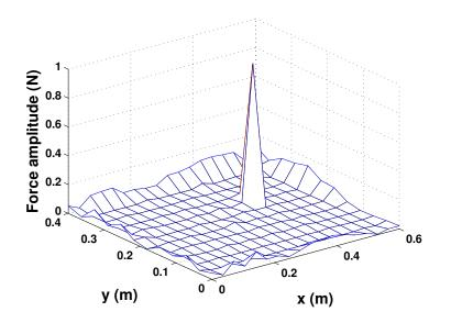
Figure 4: Reconstructed force vector  $\mathbf{F}_{\mathbf{m}}$  at 500 Hz from corrupted data using a global regularization term - q = 1.1 and  $\mathbf{L} = \mathbf{I}$
