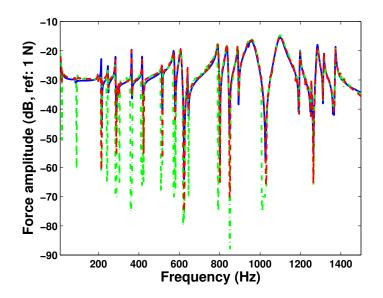
Figure 11: Reconstruction of the force spectrum - (—) Reference measured by the force sensor, (--) Multiplicative regularization and  $(-\cdot -)$  Updated additive regularization
