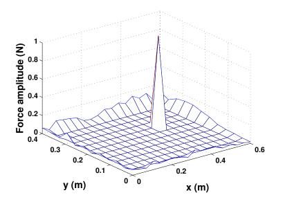
Figure 6: Reconstructed force vector  $\mathbf{F}_{\mathbf{m}}$  at 500 Hz from corrupted data when using local priors on the spatial distribution of the excitation field -  $(q_1, q_2) = (0.5, 2)$  and  $\mathbf{L} = \mathbf{I}$
