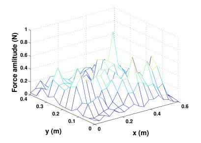
Figure 3: Naive reconstruction of the force vector  $\mathbf{F_{naive}}$  at 500 Hz
