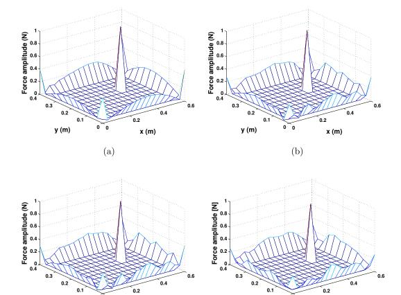
Figure 8: Comparison of multiplicative and additive regularization strategies at 100 Hz from the same corrupted vibration data, the same tuning parameters  $(q_1, q_2) = (0.5, 2)$  and the same differentiation matrix  $\mathbf{L} = \mathbf{I}$  - (a) Reference, (b) Multiplicative regularization, (c) Updated additive regularization and (d) Non-updated additive regularization
