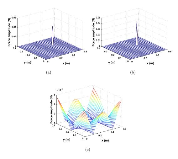
Figure 10: Comparison of additive and multiplicative regularization strategies at 196.25 Hz from the same measured data, the same tuning parameters q = 0.5 and the same differentiation matrix  $\mathbf{L} = \mathbf{I}$  - (a) Multiplicative regularization, (b) Updated additive regularization and (c) Non-updated additive regularization
