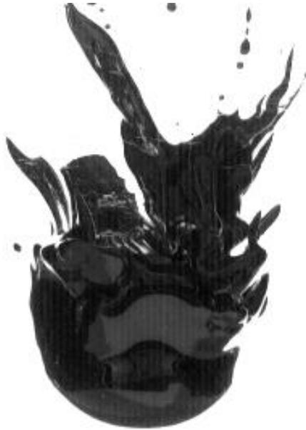
Figure 5: Snapshot of the fall of a 24 mm diapir in the most viscous ambient fluid  $R_\mu = 691$ . This corresponds to  $Re = 14$ , with  $We = 31$ ; this is an example of a diapir that does not burst although it is above the critical radius for breakup limited by surface tension (Hinze, 1955).
