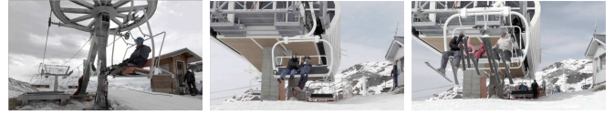
Fig. 2: Three types of hazardous user behavior (left to right: presence of passenger beyond the ski lift arrival area, bad position of passenger from the ski lift departure area, guardrail is not lowered completely beyond a given area with presence of passenger on the seat).
