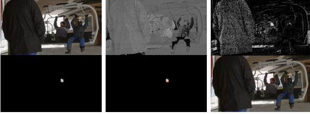
Fig. 6: Different steps of the proposed method (from left to right and top to bottom: frame_T , RGB to Hue transformation, backprojection, backprojection after applied mask, ellipse obtained by CAMshift, resulting bounding).
