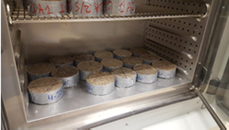
Fig. 7. The MBV samples in climatic room.
