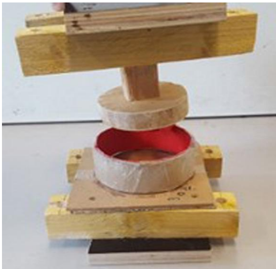
Fig. 4. Presentation of wooden molds and piston used.
