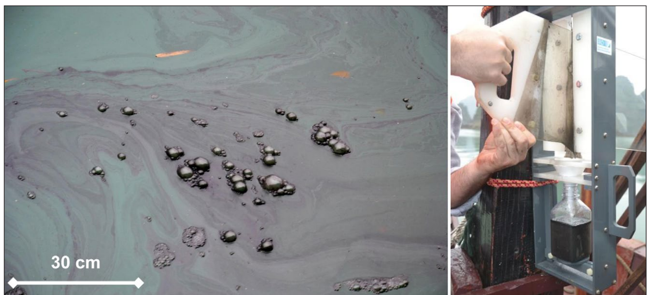
Figure 2: Black carbon slick and SML sampling. Example of a black slick observed in Halong Bay during the dry season (left), and sea surface microlayer (SML) sampling (right) using the glass plate technique within such highly BC-impacted slicks. Note the color of the SML sample; although visually resembling an oil slick in situ, analyses confirmed these black slicks were due to BC. DOI: https://doi.org/10.1525/elementa.255.f2
