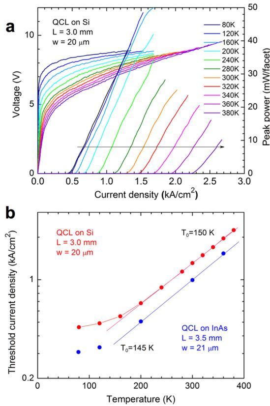
**Figure 4.** Characteristics of the studied QCLs at different temperatures. **(a)** Voltage-current and light-current characteristics of a QCL grown on Si measured between 80 and 380 K. **(b)** Threshold current density as a function of temperature of QCLs grown on Si and on InAs.
