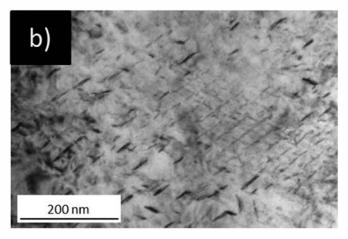
**Fig. 15.** TEM micrographs of precipitates in Ti6-4 after irradiation at 430 °C, by TEM,  $\vec{g} = 10\overline{1}1 \text{ B} \sim [1-\overline{2}13]$ : a) 0.6 dpa high flux, b) 0.6 dpa low flux.
