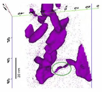
Fig. 14. Vanadium channel observed by APT analysis (isosurface V=12 at.%.) in Ti6-4 alloy irradiated at 430 °C for a dose of 3 dpa.
