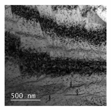
Fig. 16. TEM micrograph of a preferential precipitation on the native dislocation network.
