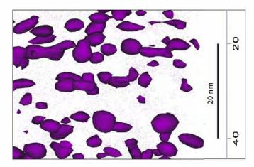
Fig. 11. Precipitates after irradiation at 300  $^{\circ}$ C for a dose of 3 dpa high flux (APT analyses). Isosurface V = 10 at.%.
