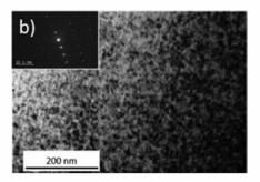
Fig. 5. <a> loops in the  $\alpha$  phase, by TEM,  $\vec{g}' = 10\overline{1}1 \text{ B} \sim [1\overline{2}10]$ , for Ti6-4 alloy irradiated at the dose of 3 dpa at high flux and at the temperature of: a) 300 °C and b) 430 °C.
