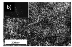
Fig. 6. <a> loops in the  $\alpha$  phase, by TEM,  $\vec{g} = 10\overline{1}$ 1 B  $\sim [1\overline{2}10]$ , for Ti6-4 alloy irradiated at the dose of 0.6 dpa and at the temperature of 300 °C: a) high flux and b) low flux.
