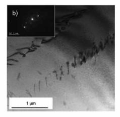
Fig. 4. TEM micrographs showing dislocation pileups:  $\vec{g} = 10\overline{1}0$  B  $\sim [1\overline{2}13]$  in Ti6-4 alloy a) as received b) after thermal treatment 6 h at 450 °C.
