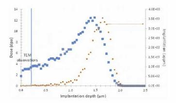
**Fig. 2.** Damage and ion implantation profiles determined from SRIM simulation for irradiations carried out with  ${\rm Ti}^{2+}$  ions at an energy of 6 MeV, using an aluminum foil degrader (0.8  $\mu$ m thick) in front of the specimens (3 dpa 430 °C high flux). The part of the profile concerned by TEM observations is indicated.
