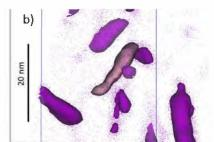
Fig. 12. Platelet-like precipitates after irradiation at 430 °C for a dose of 3 dpa high flux (APT analysis): a) top view, b) edge-on view. Isosurface V = 17 at.%.
