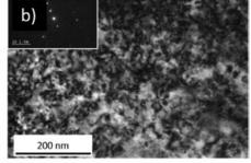
Fig. 7. <a> loops in the  $\alpha$  phase, by TEM,  $\vec{g}=10\overline{1}1$  B  $\sim$  [1 $\overline{2}10$ ], for Ti6-4 alloy irradiated at the dose of 0.6 dpa and at the temperature of 430 °C: a) high flux and b) low flux.
