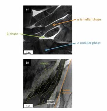
**Fig. 3.** TEM micrographs before irradiation of Ti6-4 alloy: a)  $\alpha$  nodular and lamellar phases surrounded by  $\beta$  phase and b) Dislocations forming sub-grain boundaries in nodular phase. Solid line separates the nodular  $\alpha$  phase and dotted lines the sub-grains.
