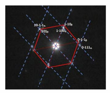
**Fig. 8.** Diffraction pattern B ~ [11 $\overline{2}$ 3]: superposition of the  $\alpha$  phase (blue dotted lines) and the  $\beta$  phase (continuous red lines) patterns. The  $\alpha$  phase corresponds to the matrix and the  $\beta$  phase to the precipitates. Sample irradiated at the dose of 3 dpa and at the temperature of 430 °C, high flux. (For interpretation of the references to colour in this figure legend, the reader is referred to the Web version of this article.)
