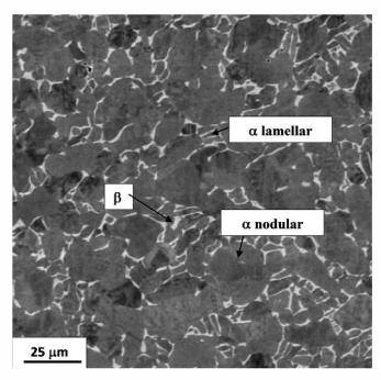
Fig. 1. BSE-SEM micrograph of the as-received Ti6-4 titanium alloy (the  $\alpha$  and  $\beta$  phases appear in grey and white, respectively).
