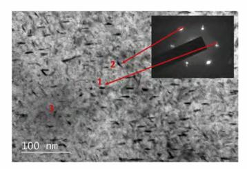
**Fig. 9.** TEM micrograph of radiation-induced precipitates into the  $\alpha$  phase, B ~ [11 $\overline{2}$ 3], in Ti6-4 alloy after irradiation at 430 °C for a dose of 3 dpa high flux.
