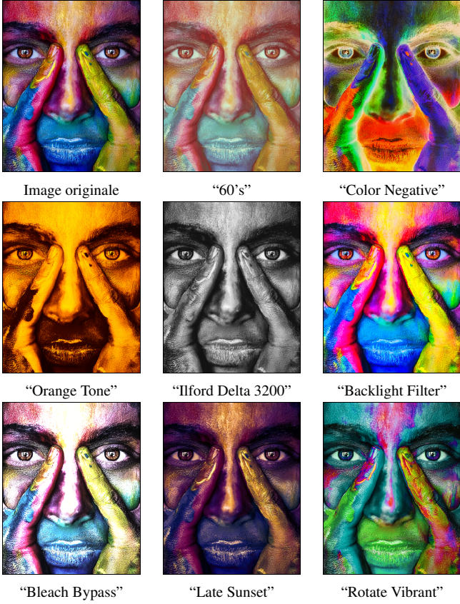
FIGURE 2 – Generic nature of color transformations allowed by the use of 3D CLUT s.
