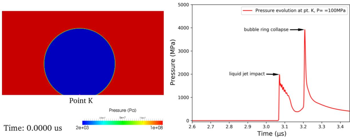
Figure 3a (left) : Initial bubble setup with represented point  $K$  in the bottom solid boundary where pressure evolution is plotted; Figure 3b(right): Pressure evolution at point  $K$  in the bottom solid boundary,  $R_{max} = 500 \mu m$ ,  $\gamma = 0.8$ ,  $P_{\infty} = 100 MPa$
