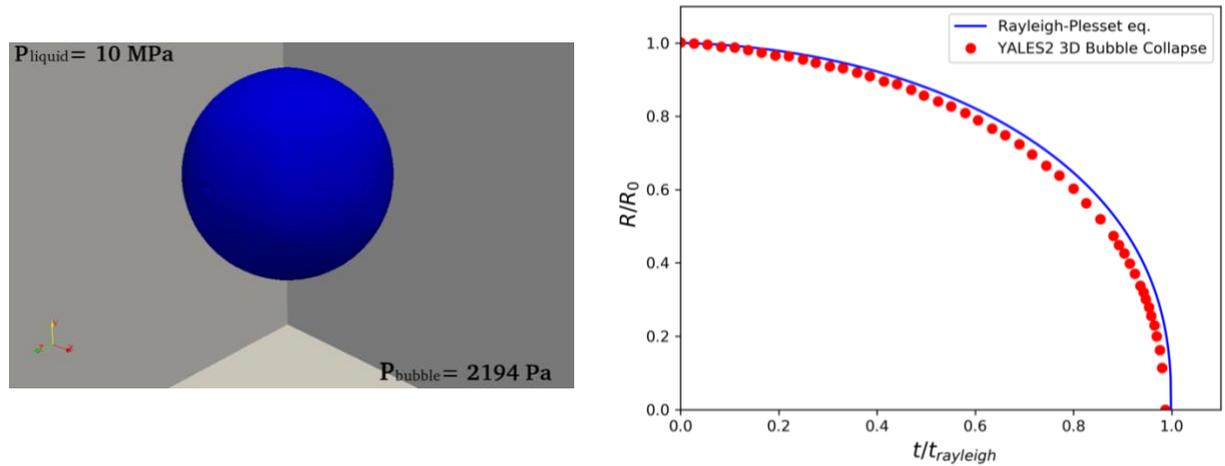
Figure 2 : Simulation of a single 3D spherical bubble collapse with YALES2 and comparison with Rayleigh Plesset collapse model for  $R_{max} = 500 \mu m$ ,  $P_{\infty} = 10 MPa$ . Numerical bubble collapse setup (left); evolution of non-dimensional radius with respect to non-dimensional time (right)
