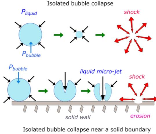
Figure 1: Vapor bubble collapse due to imposed pressure difference  $P_{liquid} \gg P_{bubble}$ ; collapse of an isolated bubble - symmetric collapse (top); bubble collapse near a solid boundary - asymmetric collapse (bottom)
