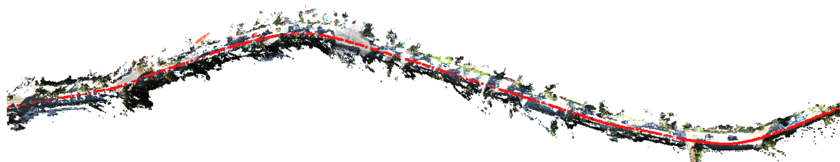
Figure: reconstructed point cloud correctly fitting the GPS coordinates (in red).
