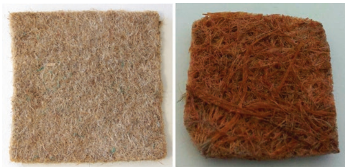
Fig. 1.8 Hemp felt before ( left ) and after adsorption ( right ) in a solution containing a mixture of six metals
