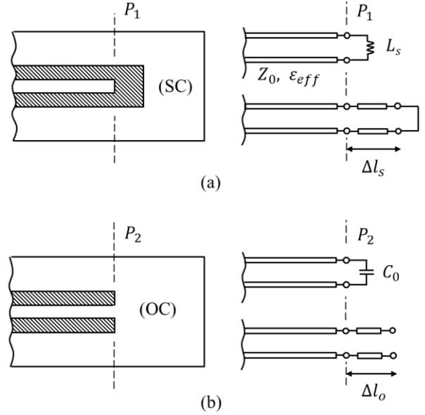
Fig. 2. Physical CPS discontinuities and their models. (a) Short circuit modeled either by a lumped inductance  $L_s$  or by an additional TL section of length  $\Delta l_s$ . (b) Open circuit modeled either by a lumped capacitance  $C_0$  or by an additional TL section of length  $\Delta l_o$ .
