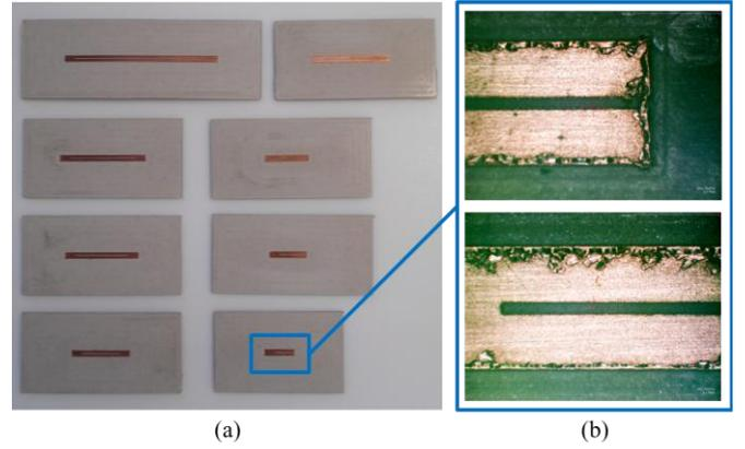
Fig. 4. Pictures of the realized scatterers of the series n°1. (a) Pictures of the 8 realized scatterers: 4 loop and 4 C-like. For each couple of scatterer, the length of the strips is chosen such that  $l_A = 2l_B$ . (b) Expanded view of a C-like scatterer.
