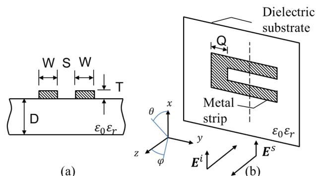
Fig. 1. (a) Transverse section of coplanar stripline (CPS). (b) RCS measurement principle. A resonator that incorporates the discontinuity to be tested is illuminated by a plane wave  $E^i$ . The backscattered field  $E^s$  is measured.
