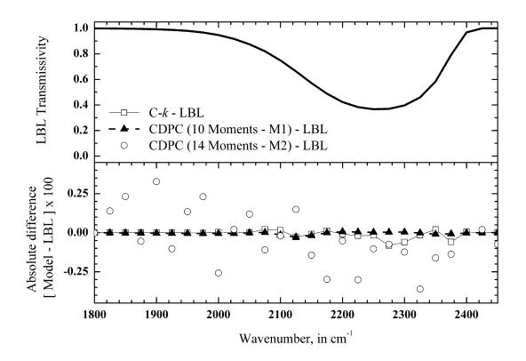
Figure 3. Narrow band (25 cm<sup>-1</sup>) transmission function for 10 cm of 10 % CO<sub>2</sub> – 90 % N<sub>2</sub> at 2900 K and 1 atmosphere – Top: LBL reference calculation. Bottom: absolute difference x 10<sup>2</sup> between LBL and approximate models (C-*k*, CDPC with methods M1 and M2).
