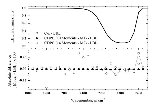
**Figure 2.** Narrow band (25 cm<sup>-1</sup>) transmission function for 10 cm of 10 %  $CO_2 - 90$  % N<sub>2</sub> at 1500 K and 1 atmosphere – Top: LBL reference calculation. Bottom: absolute difference x  $10^2$  between LBL and approximate models (C-*k*, CDPC with methods M1 and M2).
