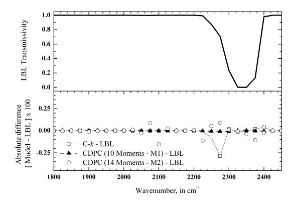
Figure 1. Narrow band (25 cm<sup>-1</sup>) transmission function for 10 cm of 10 % CO<sub>2</sub> – 90 % N<sub>2</sub> at
