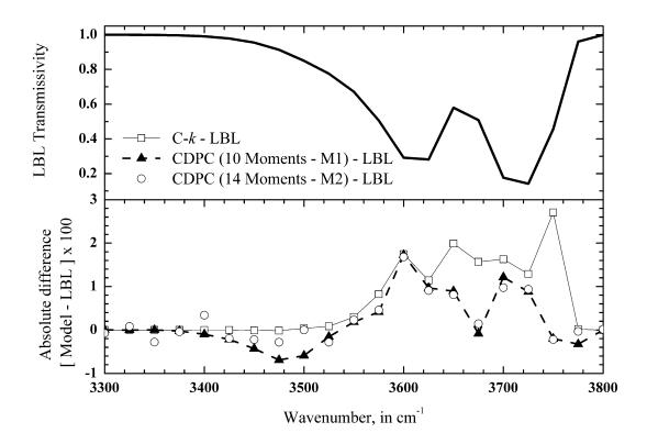
Figure 6. Narrow band (25 cm<sup>-1</sup>) transmission function for a non-uniform path (see text for details) – Top: LBL reference calculation. Bottom: absolute difference x 10<sup>2</sup> between LBL and approximate models (C-*k*, CDPC with methods M1 and M2).
