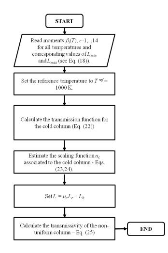
Figure 5. Flowchart for the application of the CDPC approximate model in non-uniform
