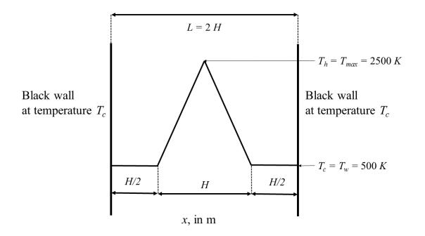
**FIGURE 7.** Triangular temperature profile considered for the comparison of the SLW model with the reference approach described in Ref. [2], RC-SLW model Ref. [5] and LBL calculations.
