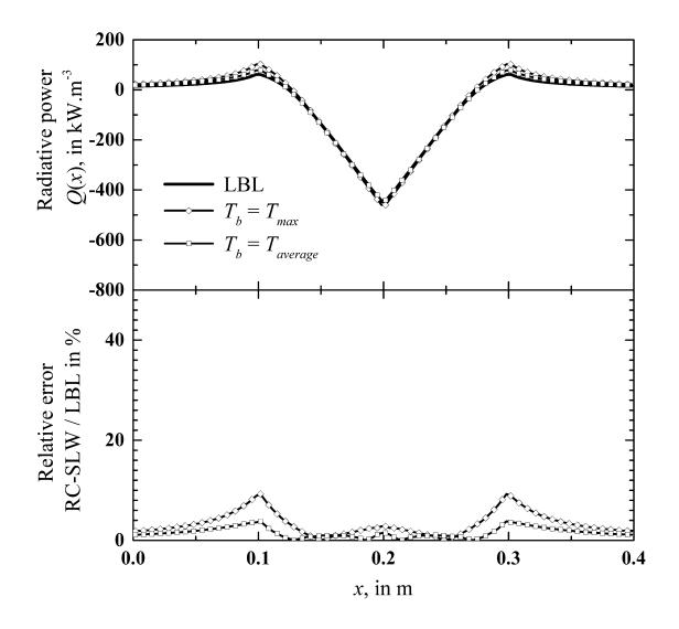
**FIGURE 9.** Comparison of the RC-SLW [5] model with LBL reference calculations. Triangular temperature profile of Figure 7 ; H<sub>2</sub>O-N<sub>2</sub> mixture ( $x_{H2O} = 0.1$ ) at atmospheric
