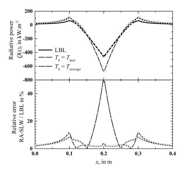
**FIGURE 8.** Comparison of the SLW model with the reference approach of Ref. [2] (RA-SLW) with LBL reference calculations. Triangular temperature profile of Figure 7; H<sub>2</sub>O-N<sub>2</sub> mixture ( $x_{H2O} = 0.1$ ) at atmospheric pressure. Relative errors are calculated as
