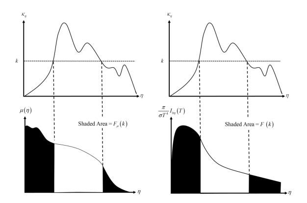
**FIGURE 2.** Definition of functions  $F_{\mu}$  and F.
