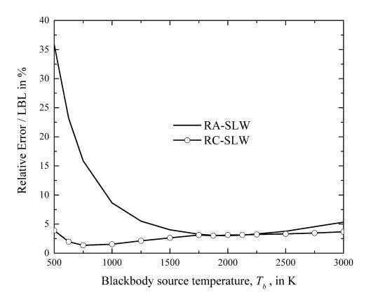
FIGURE 10. Relative errors of the RA-SLW and RC-SLW models for different blackbody
