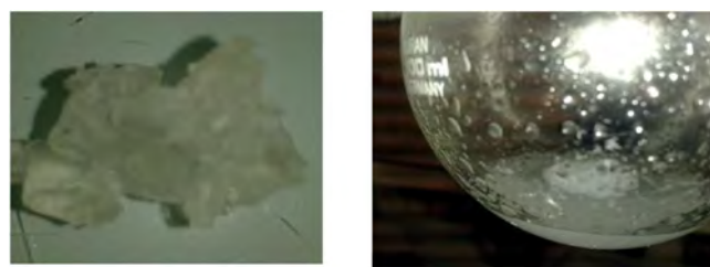
Fig. 2. (left) PDMDMA homopolymer obtained in solvent-free conditions, (right) viscous liquid obtained in the flask after synthesis in THF (magnetic stirring) and evaporation of the solvent.
