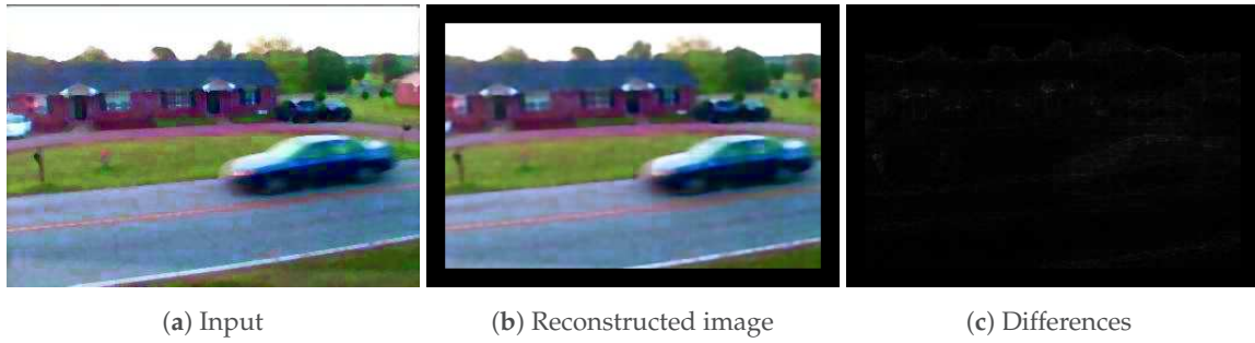
Figure 1. Reconstruction using an autoencoder. We trained the autoencoder using patch images as reference images. We cropped patch images for a current image in (a) and reconstructed each patch in (b). It is difficult to select a threshold value to distinguish the foreground clearly using the differences, as shown in (c).
