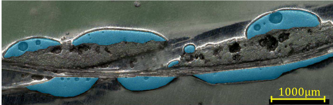
Figure 1. Semipreg fabric cross-section; the PA66 droplets are highlighted in blue
