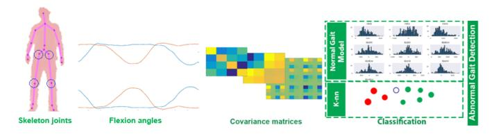
Fig. 1. The proposed binary gait assessment pipeline. We select the most stable among low-limbs skeleton joints to calculate flexion angles. Then the angles-based covariance features are used for gait assessment in different scenarii.
