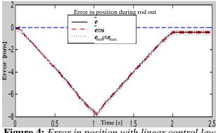
Figure 4: Error in position with linear control law
