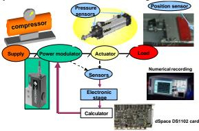
Figure 1: Principle of electropneumatic system.
