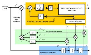
Figure 2: Principle of nonlinear tracking control.
