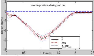
Figure 5: Error in position with nonlinear control law
