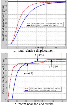
Figure 3: Step response with scheduled and fixed gains near the stroke extremity.
