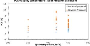
Fig.2 Distribution graph of variation of spray temperature (Ts) of TiO<sub>2</sub> layer prepared by using propanol as a solvent and PCE of perovskite solar cell.
