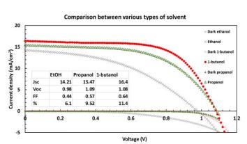
Fig.1 Comparison of J-V curve from various types of solvent.
